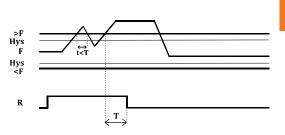
M: with memory means if fault occur only for one time, relay c/o can not return to normal status automatically, unless power supply restart
