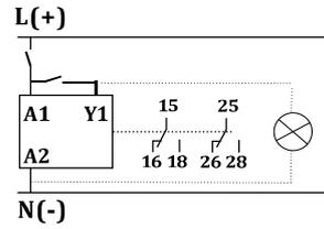
Note: If A1-A2 is DC power supply, A1 must be positive, A2 must be negative
